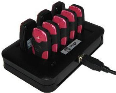
Figure 2.4.2-1: Faros sensor on charger station
